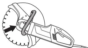
When the blade is replaced with a new one, check the flange washers and the drive axle. See instructions under the heading Checking the drive axle and flange washers.
