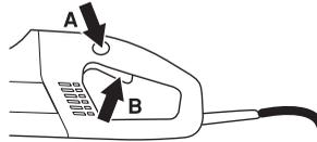
The power switch lock remains depressed as long as the power switch is depressed. When the grip on the handle is released both the power switch and power switch lock are reset. This movement is controlled by two independent return springs. This position results in the machine stopping and the power switch being locked.
