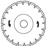
There is an arrow on the machine that indicates the axle's direction of rotation that the blade is mounted on.
