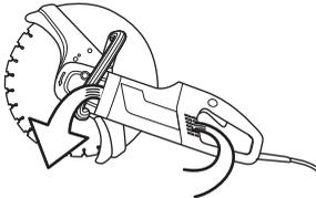
In order for the machine to always be cooled sufficiently the cooling air openings must be kept clear and clean. Blow down the machine regularly with compressed air.
