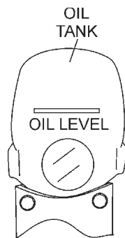
Figure 7. Oil Tank (Front View)
