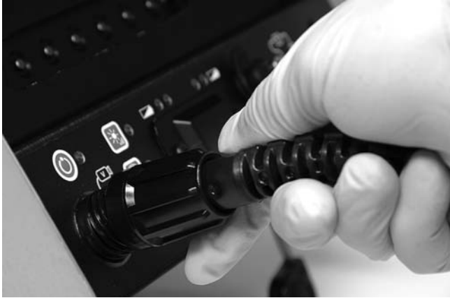
Figure 13 – Connecting To A SeeSnake CCU
