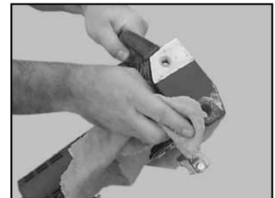
(I) Clean the Cutting Head Pivot Holes
