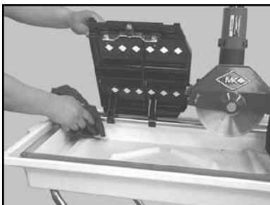
(A) Check that the Guide Bar is clean – clean if dirty
