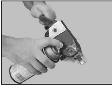
(J) Lubricate the Cutting Head Pivot Holes
