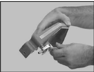
(G) Remove the Blade Guard Intake Fitting
