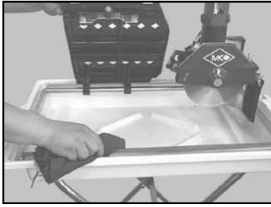
(J) Clean the Roller Wheel Guide Rail
