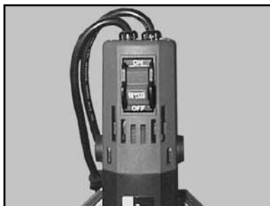
(K) Turn the motor OFF when work is complete
