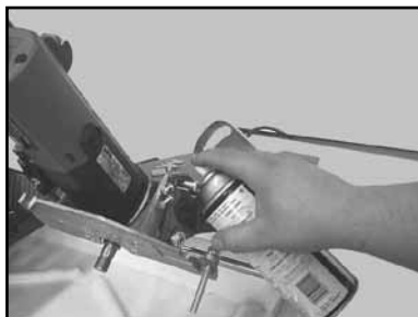
(G) Lubricate the rear Cutting Head Pivot Point
