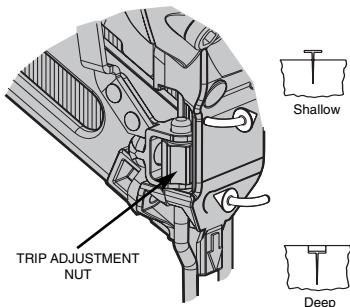
The DIAL-A-DEPTH™ Fastener Control adjustment feature provides close control of the fastener drive depth; from flush with the work surface to shallow or deep countersink. First, set the air pressure for consistent drive in the specific work as described on page 4, then use the DIAL-A-DEPTH™ Fastener Control adjustment to give the desired depth of drive.
